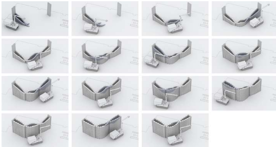
Fig. 7. Simulation of one possible building sequence of the wall's construction: The double-leaf brick wall with the dimensions of 6.5m length and 2m height, consisting of 1600 bricks, is subdivided to be fabricated from 15 different positions of the mobile robot.
