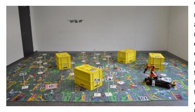
We face a scenario where a ground robot must deliver an emergency kit to a victim, which is too heavy for a flying robot. To find the victim and spot obstacles on the way, the flying robot can exploit its bird's-eye view. A mission plan is computed that includes the removal of small obstacle. Then, the flying robot guides to ground robot to the victim and monitors the mission. All steps are executed without any human intervention. This demo was
