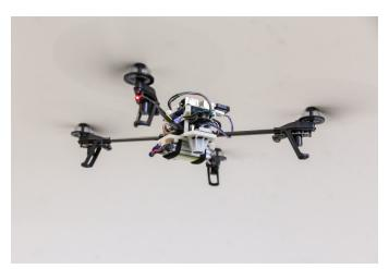
Our quadrotors can navigate autonomously without any external infrastructure: all sensing and computation is done onboard. We use vision as main sensing modality and process the images on a smartphone computer. This allows the quadrotor to navigate in GPS-denied environments, with lacky communication links, and without any human intervention. Our 3D reconstruction software allows to build a map of the
